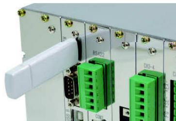
The USB host port is installed in CPU substrate of this unit. Data between PC can be handed over by using USB thumb drive. When maintaining it, it can back up data, and the program can be updated.
